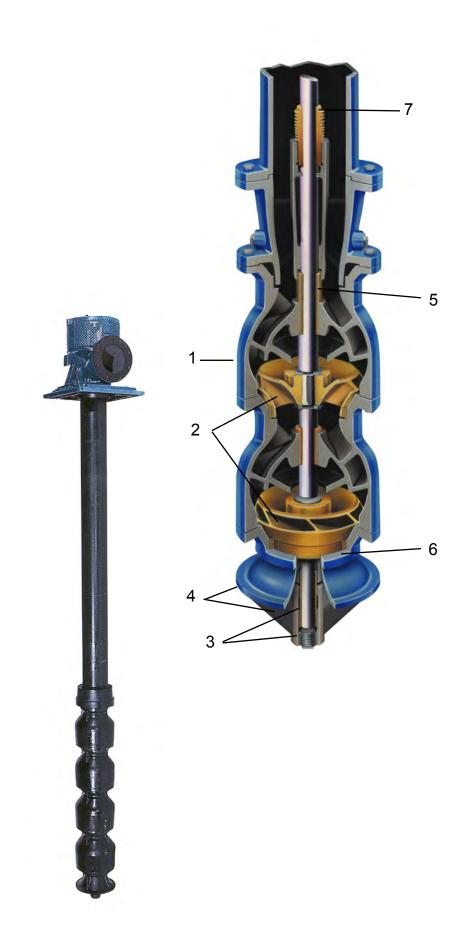
1. Bowl castings are manufactured of heavy-duty, high quality cast iron, and feature a minimum 30,000 PSI tensile strength, with smooth passages designed for efficient operation. Optional coated passages are available to further pump efficiency. Bowls can be staged to produce higher pressures for a given capacity. (Threaded bowl connections are used in the 6M, 7M and 8M designs.)
