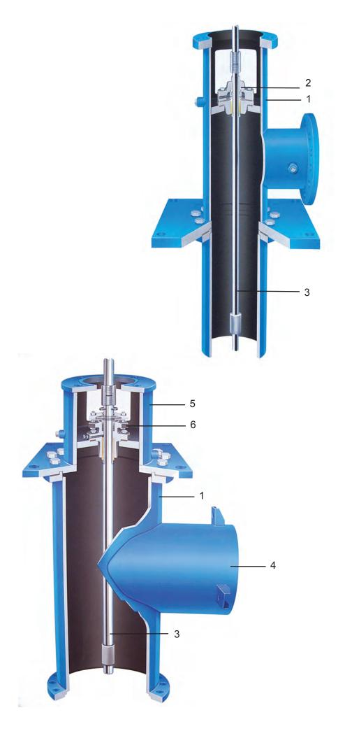
1. The L-type fabricated discharge heads are designed to accept the column, shaft, and bowl weight as well as the hydraulic thrust. The heads are formed from high quality steel and gusseted providing a rigid base to eliminate vibration and assure smooth operation. Plain-end and flanged discharge designs are available through 300 lb. flange ratings.
