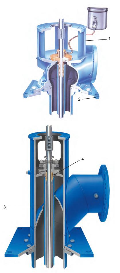
1. Rugged cast iron discharge heads meet sanitary requirements and support the column, lineshaft, and bowl assemblies, while accepting any vertical driver. Large openings allow easy access to the stuffing box or mechanical seal, and smooth passageways ensure reduced friction loss and efficient overall operation. The integrally-cast discharge flange can be either a 125 lb. or 250 lb. design.
