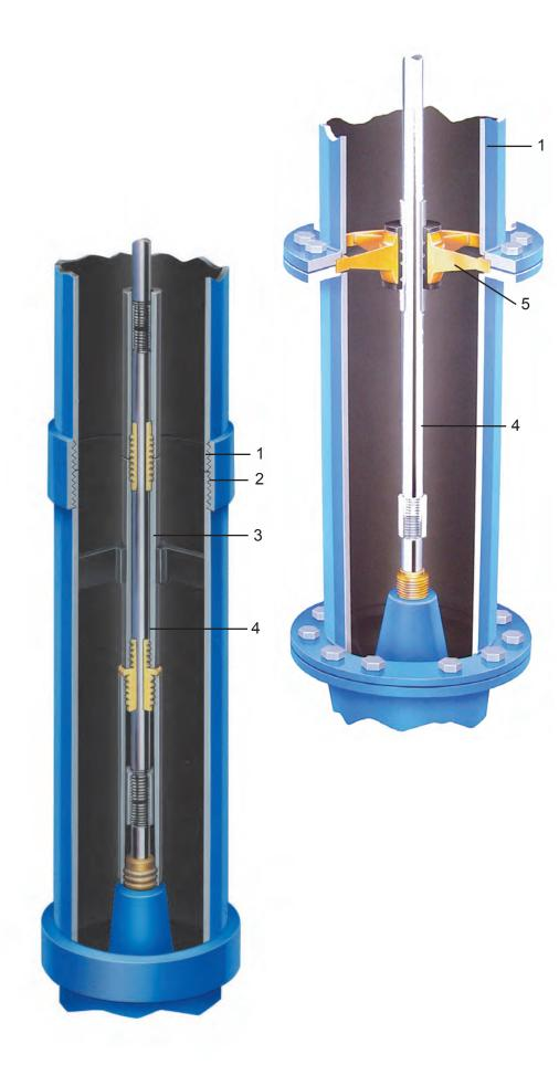
1. Threaded steel discharge column is available in standard sizes through 14" diameter. Where greater strength or ease of assembly and disassembly is required, flanged column pipe is also available in these sizes. Welded flanged column is supplied as standard in column sizes 16" and larger.
