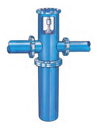
To meet unique requirements, vertical turbine pumps can be incorporated with a "pot" or "can". These units are typically found in applications where the Net Positive Suction Head Available (NPSHA) is low, in high pressure systems, systems where suction pressures are variable and/or critical, or where differences in the elevation of suction and discharge piping is desired.
