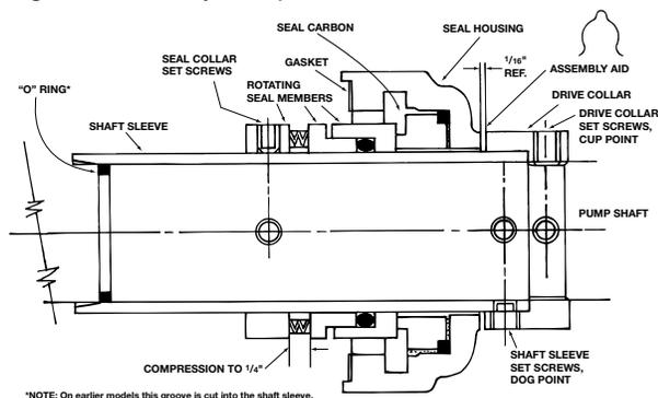
\*NOTE: On earlier models this groove is cut into the shaft sleeve.
