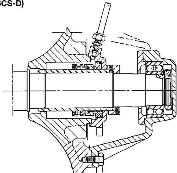
17. Compress rotating seal assembly to a 1/4" space between the seal parts that house the compression springs. Tighten set screws.
