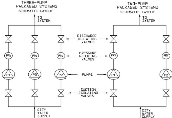
Figure 2. BOOSTER PIPING ARRANGEMENTS
