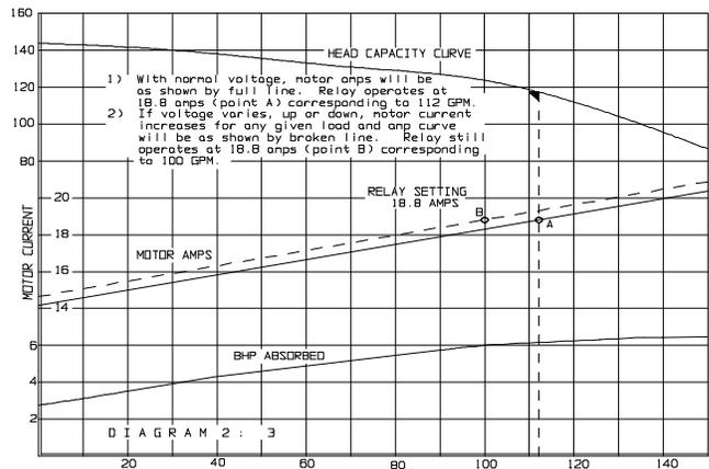
Figure 1. CURRENT SENSING DIAGRAM
