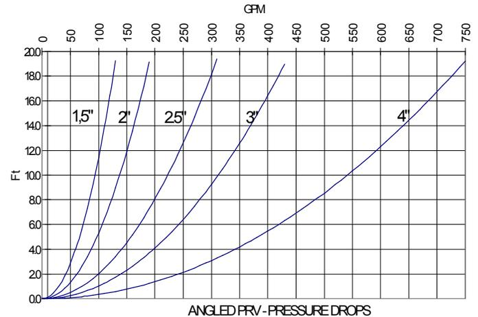
Figure 5. PRV PRESSURE DROP CHART
